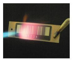
Laser Engraved Ceramic On Stainless Steel offers the option of printing information onsite using a compatible YAG or CO<sup>2</sup> laser or they can be preprinted at Metalcraft. These labels provide excellent durability against high temperatures and chemicals. Possible applications include work in process tracking for automobile parts and identification tags for airplane components and steel companies.
